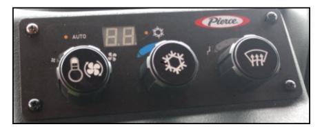
The system will control the temperature of the cab and crew cab automatically by pushing the center of the fan speed control knob. Rotate the center temperature control knob to set the cab and crew cab temperature.
