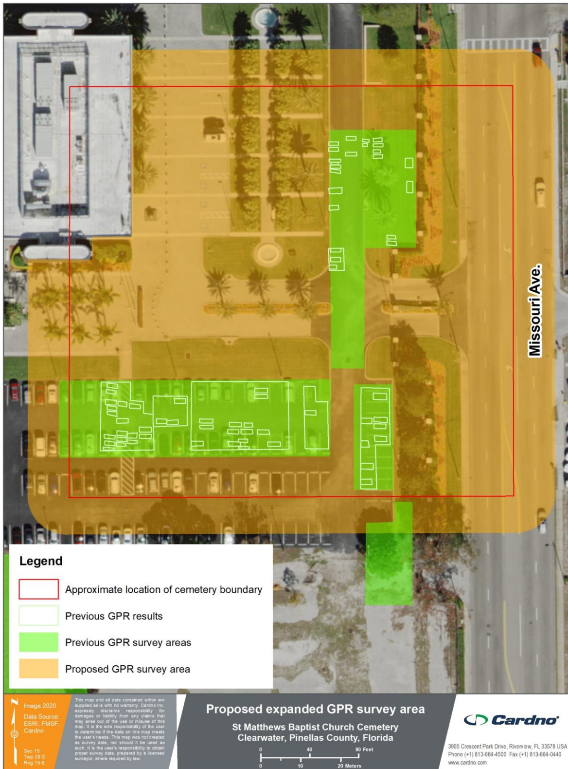
Figure 45 Proposed expanded GPR survey area to determine land-use boundaries of cemetery
