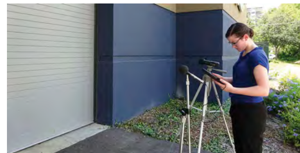
Figure 11. Acoustical measurements and recordings of sound propagating through the roll-up doors at an existing facility similar to the proposed central energy plant.
