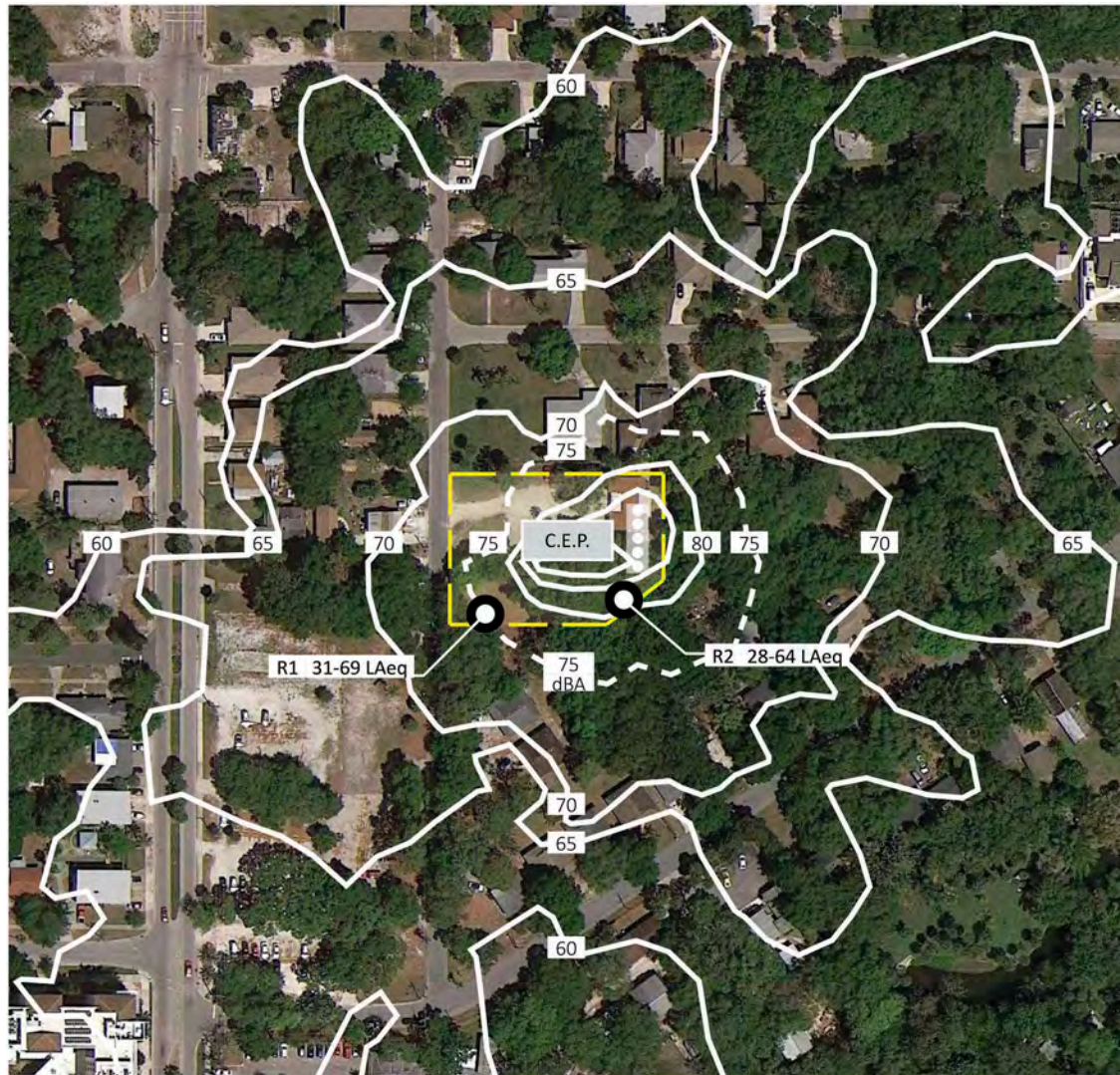
Figure 2. Sound contour map showing that the noise generated from the proposed chiller plant exceeds the city's noise ordinance (75 dBA) and measured ambient sound levels (locations R1 and R2). The computer model included five cooling towers within a sound-absorbing enclosure; the chiller building consisted of a concrete roof, CMU walls, regular roll-up doors, typical man doors, three chillers and six pumps, and interior sound-absorbing material.
