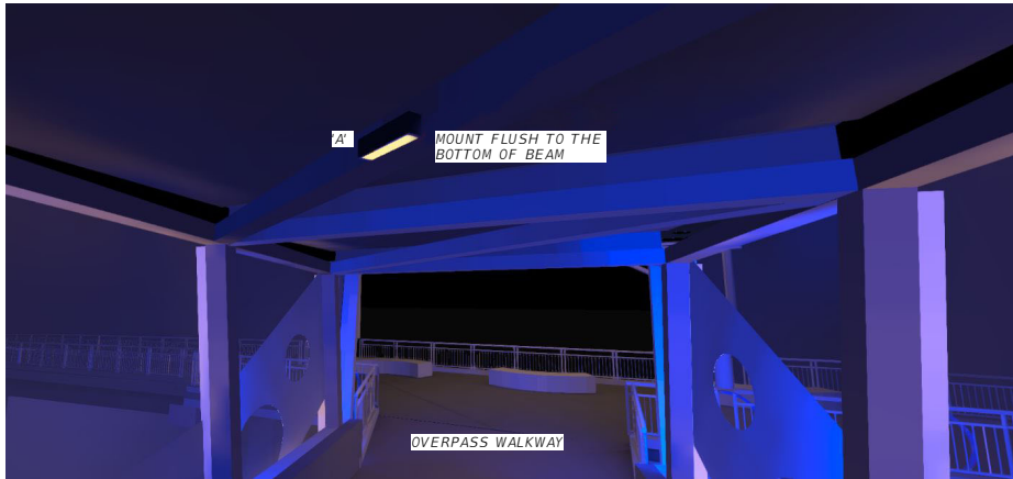
1 LUMINAIRE TYPE 'A' MOUNTING DETAIL
