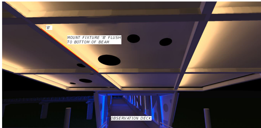
2 LUMINAIRE TYPE 'B' MOUNTING DETAIL
