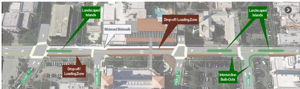
Figure 29: Concept Plan Removing Northbound Left Turn Lane at Pierce Street
